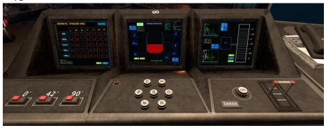
**Work Order:** The work order is located on the control desk in the control room. It specifies the grade of steel that the user will be producing in the simulation and will detail the quantity of each element required for that steel.
