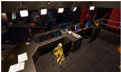
**Location 2 - Cabin**: The cabin is the second location in the simulation and it is where the user will be able to control three large machines used in the steel production process. The cab is above the basic oxygen furnace. The user will be able to control the magnet crane used for unloading scrap metal into the scrap box, scrapbox which is used to unload the scrap metal into the oxygen furnace and an iron ladle which can pour in the molten iron into the scrap box.
