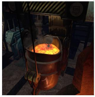
**Iron Ladle Screens:** When the iron ladle is being controlled by the cabin, the two screens above the user will display helpful information about the iron ladle. The left screen will display the tilt angle of the oxygen furnace, which will need to be at 42 degrees to add the molten iron. The right screen will display the location of the iron ladle relative to the oxygen furnace as well as indicators of where the user will need to move the iron ladle.
