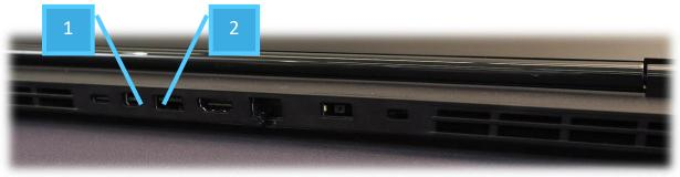
**NOTE:** The DisplayPort cable (1) has a Mini DisplayPort adapter on the end of it that is needed to connect your headset to the laptop. If you lose or damage this adapter, replacements are available online.
